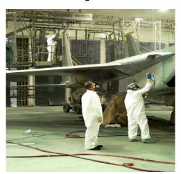
aircraft exteriors, interiors or parts. Exposure can also occur during the stripping of paint in preparation for a new coating.
